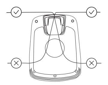
The entire charging station must be inside the operating area as shown in the figure.
