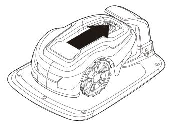
Place the mower into the charging station while the boundary and guide wires are being laid.
