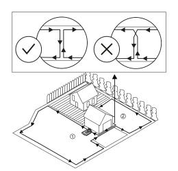
Temporarily secure the end of the loop wire to a peg or other object at the charging station.
