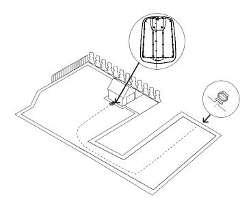
The mower uses the optional guide wire to find its way back to the charging station, but also find hard-to reach areas of the operating area. For example, the guide wire is laid between the charging station and a remote part of the working area or through a narrow passage.
