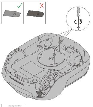
WARNING! Press the STOP button and remove the safety key before replacing blades and wear protective gloves. WARNING! Use only GLOBE'S blade: 333092355
