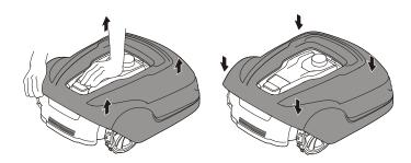
Hold down the mower with one hand and lift firmly at one of the corners of the body and repeat for all four corners, until the body pops loose from the chassis.
