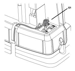
Insert both ends of the boundary wire as well as the end of the guide wire into the splice and guide wire connector. Check that the wires are fully inserted into the splice and guide wire connector so that the ends are visible through the splice and guide wire connector.
